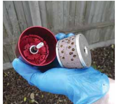
Ensuring fuel is delivered to the appliance without containments or restrictions to flow - the importance of oil supply filters should not be understated
