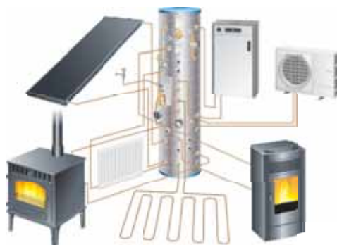
This schematic shows how a variety of fuels and renewables can be connected to the HEATBANK Xcel from Specflue
