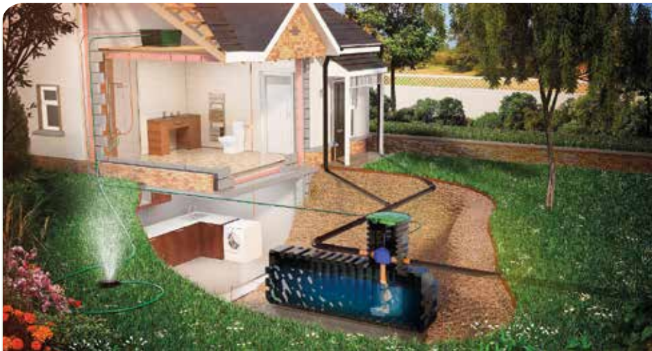
A cut-away illustration showing how the Kingspan Gamma tank can work
