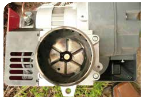
A burner from the NI field trial in 2012 showing no soot or carbon deposits on burner or combustion head.
