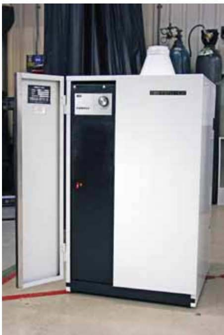
The 1960s Firefly oil-fired boiler which now stands in the museum
