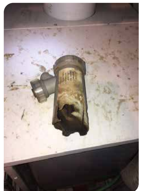
Hidden away under a slate – the fire valve of an old Heatslave boiler
